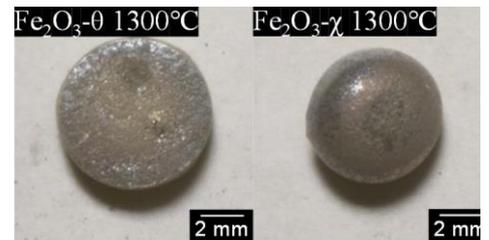
Fig. 3 Appearances of  $\text{Fe}_2\text{O}_3\text{-}\theta$  and  $\text{Fe}_2\text{O}_3\text{-}\chi$  before and after heated up to  $1300^\circ\text{C}$
